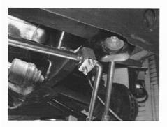
With the anti roll bar fitted, the car should be positioned on level ground so that the preload on the drop links can be set. These are adjusted so that there is no twisting load on the bar with the car suspension on level ground
