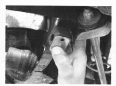
Position poly blocks as shown, checking there is sufficient clearance between roll bar and tie rod mounting bracket.
