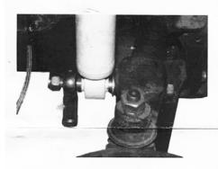
With the roll bar mounted, the drop links can be fitted to the top wishbone using the longer 5"x 3/8UNF" bolts supplied. If coil over dampers are fitted, the alloy spacers supplied are used to space the rod ends away from the wishbone where the damper would fit.
