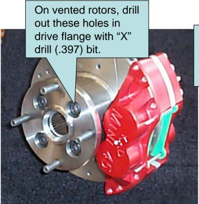
Chamfer brake pads to clear caliper spacers
